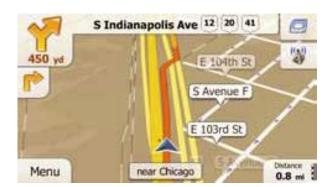
There is a field in the top left corner that displays the next maneuver. Both the type of the event (turn, traffic circle, exiting freeway, etc.) and its distance from the current position are displayed.
